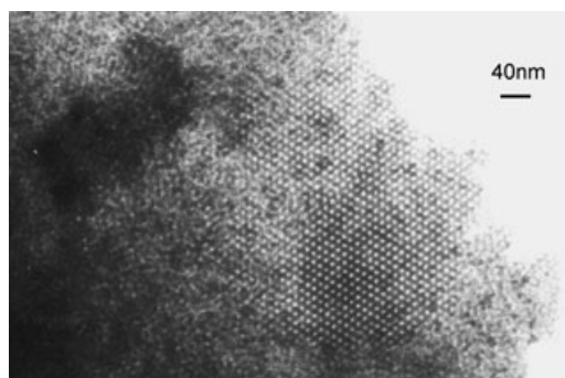
Figure 3. TEM image of the \text{CeO}_2 nanostructured material after calcination at 500^\circ\text{C}
